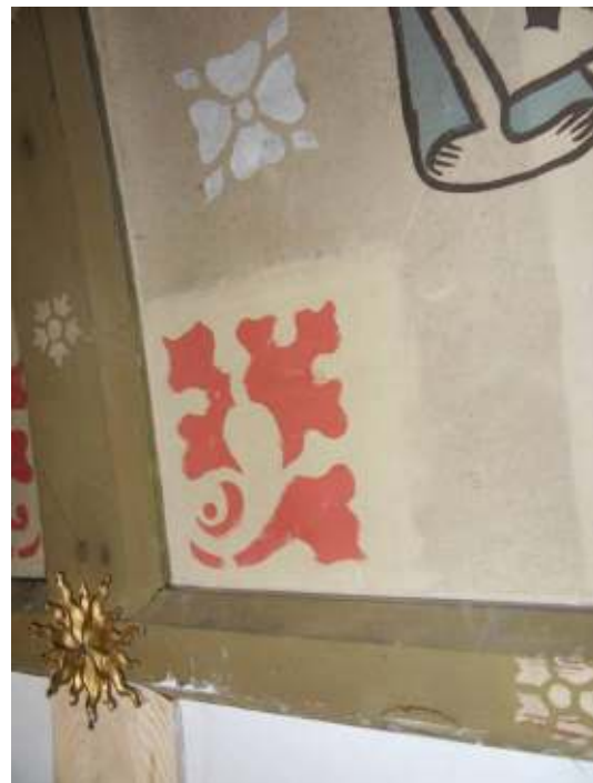
Figure 39: Detail of area of cleaning trial using a Wishab sponge.
